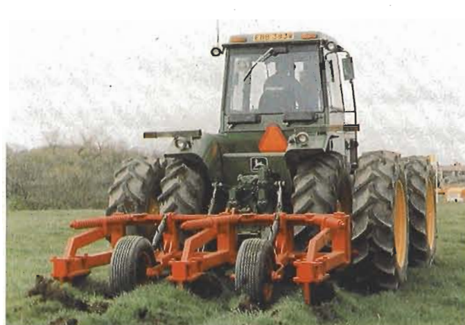
Fig. 20. A subsoiling plough at work, breaking up compacted layers below the topsoil.
