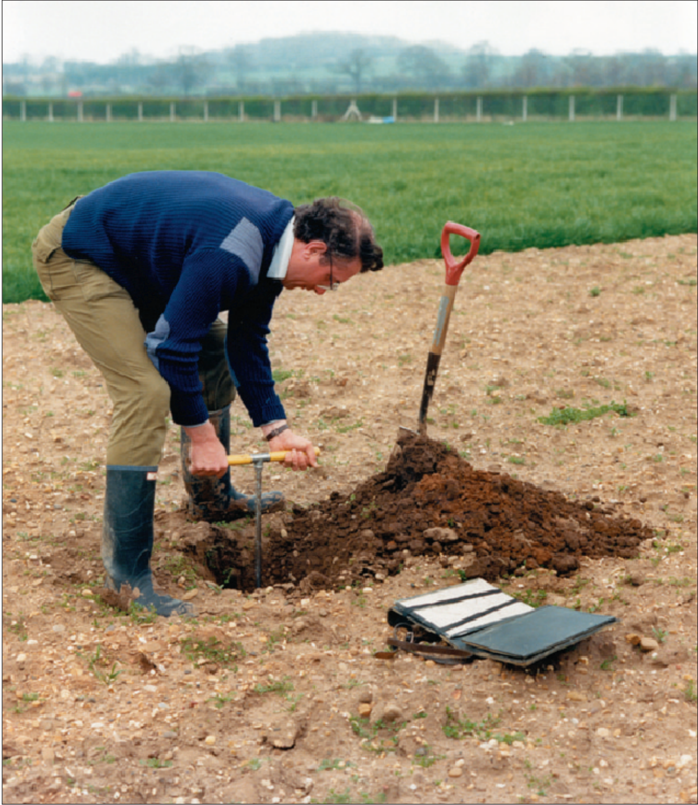
Traditional soil mapping is conducted by inspecting the soil with an auger and spade at intervals throughout the landscape. The intervals between inspections can be according to a pre-determined grid or, more often, based upon the judgement of the surveyor who uses his or her knowledge of the relationship between soil type and landscape, geology and vegetation to determine where to make inspections. Auger borings are supplemented by excavated profile pits at determined points in the landscape where boundaries between soil types occur (JH).
