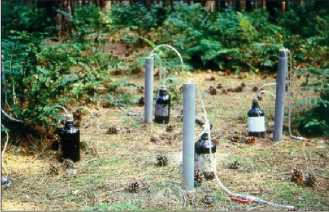
Special instruments known as lysimeters have been positioned in the forest to collect data on the amount and the chemical composition of soil water at different soil depths (EVR).
