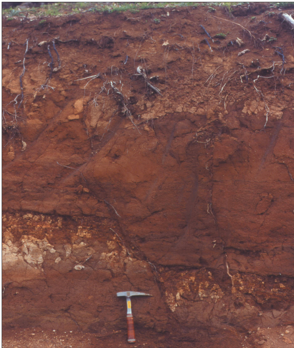
Soil is able to preserve evidence of past seismic events. This picture shows a recent normal fault cutting a soil profile on andesitic tephra near Rome. The soil on the right of the fault has dropped approximately 30 cm with respect to the in-situ material on the left (GM).
