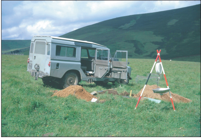
More detailed investigations in the field include weighing soil fractions to calculate stoniness (RJ).
