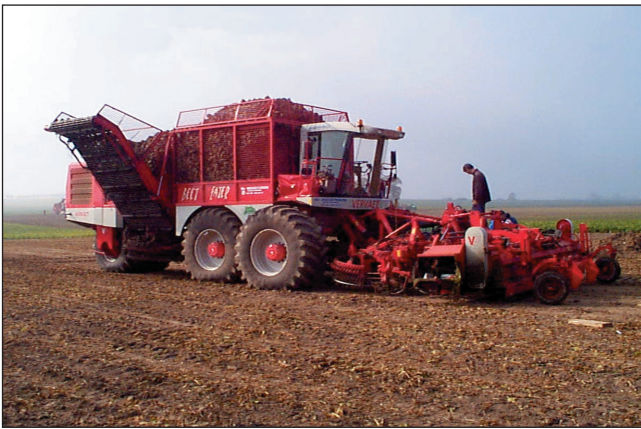
Areas degraded by soil compaction are increasing because wheel loads in agriculture are still increasing. Twenty years ago wheel loads of 50 kN (5000 kg) were considered very high. Nowadays wheel loads of up to 130 kN are used during the harvesting of sugar beet. Modern self-propelled slurry tankers with injection equipment with wheel loads of 90 – 120 kN are used in early spring on wet soils. Large tyres with an inflation pressure of about 200 kPa are needed to carry such high wheel loads. Even on moderate strong soil, compaction of up to 80 cm below the surface have been measured under such loads. The result is that the soil is increasingly compacted to ever-greater depth. The conclusion is that European soil is more threatened than ever (JJHVDA).
