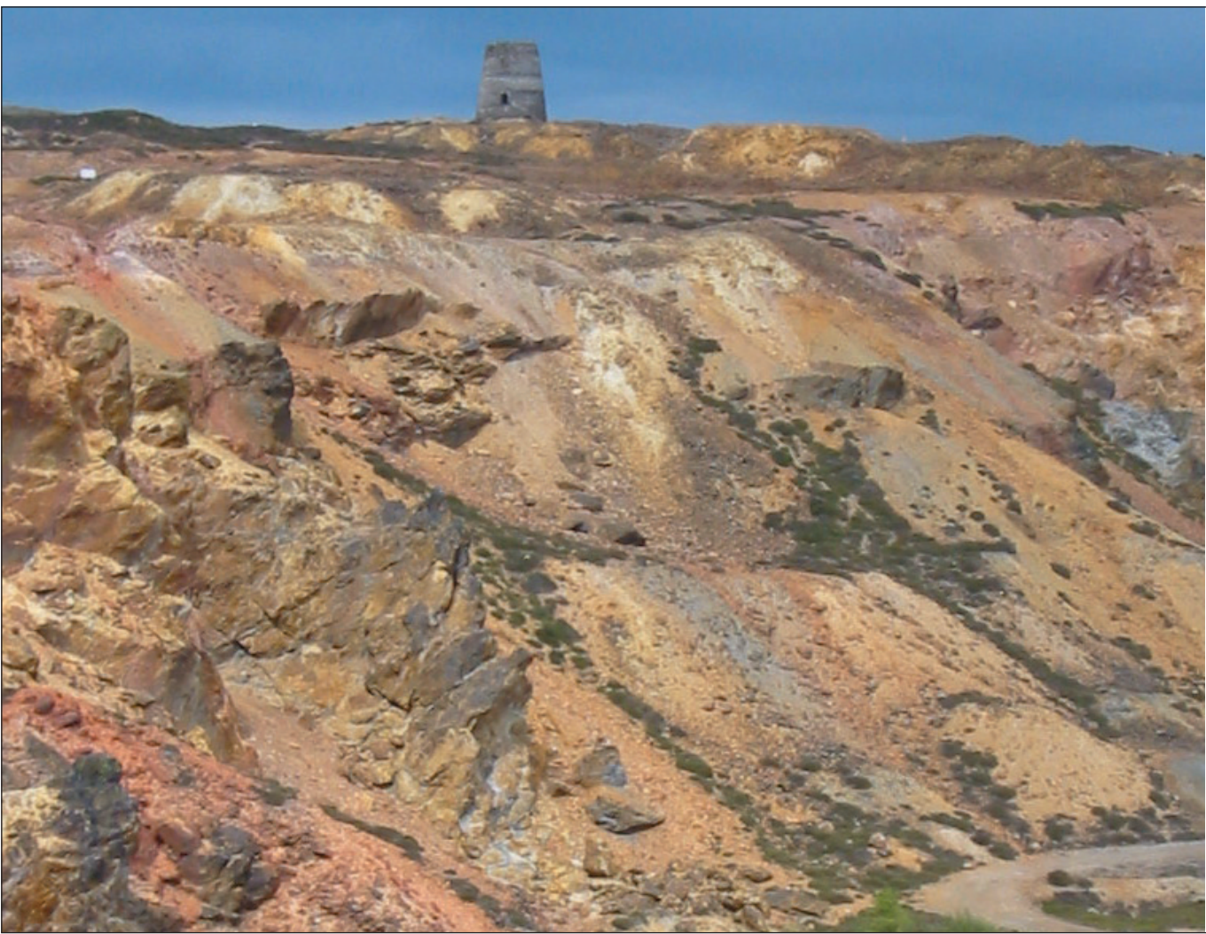
The risk of soil contamination from mining activities is associated with the storage or disposal of tailings, acid mine drainage and the use of certain chemical reagents in the processing of metal ores. This striking photograph shows an old copper mine in the UK more than 100 years after the mine was abandoned. Notice the lack of vegetation on the soil heaps. The pH of some of the old tailing ponds can be as low as 2.5, strong sulphuric acid! (AJ).
