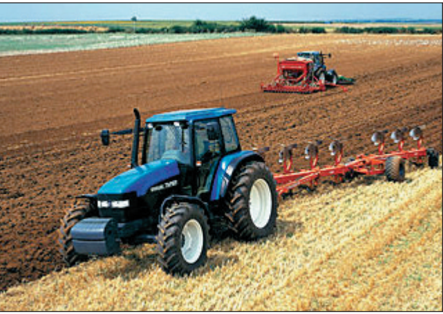
Driving heavy tractors on the subsoil during ploughing and harvesting is a major cause of subsoil compaction. The picture clearly shows how the wheels on one side of the tractor are driven in the plough furrow and press directly on the subsoil (JJHVDA).
